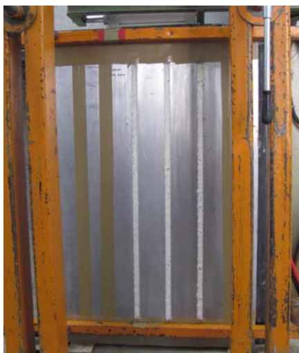
Fig. 1 Joints gunned with foam in test apparatus for linear joints according to DIN 18542, mounted in window test rig
